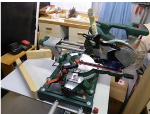
Photo 3: The base sheet extends out the back of the saw to accommodate the extent of the saw slide. Two boards (the lower frame of the shroud) were fixed to this sheet in a v shape to channel
