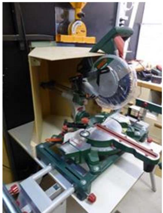
Photo 5: The top extends over the front of the saw with a cut-out to accommodate the handle. The width of this cut-out reflects the position of the
