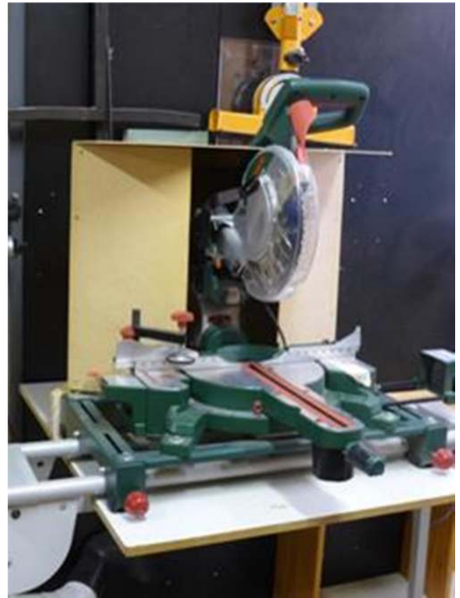
Photo 9: The finished shroud (at least for now). The shroud is doing a reasonable job in capturing a lot of the dust especially with narrow planks. With wider planks the saw is extended well in front of the shroud and a lot of material is thrown out on the right hand side of saw blade before it enters the shroud.
