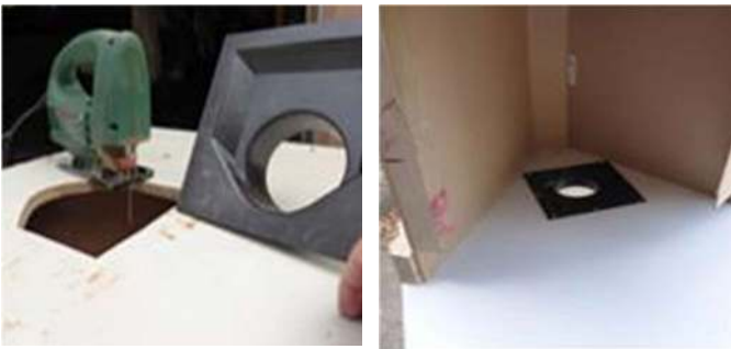
Photos 6 & 7: Cut-out for inserting the 100 mm dust extractor connector in the back and bottom of the shroud.
