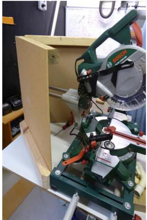
Photo 4: Light fibre board was used for the walls; the flat top and back (also see next photo.
