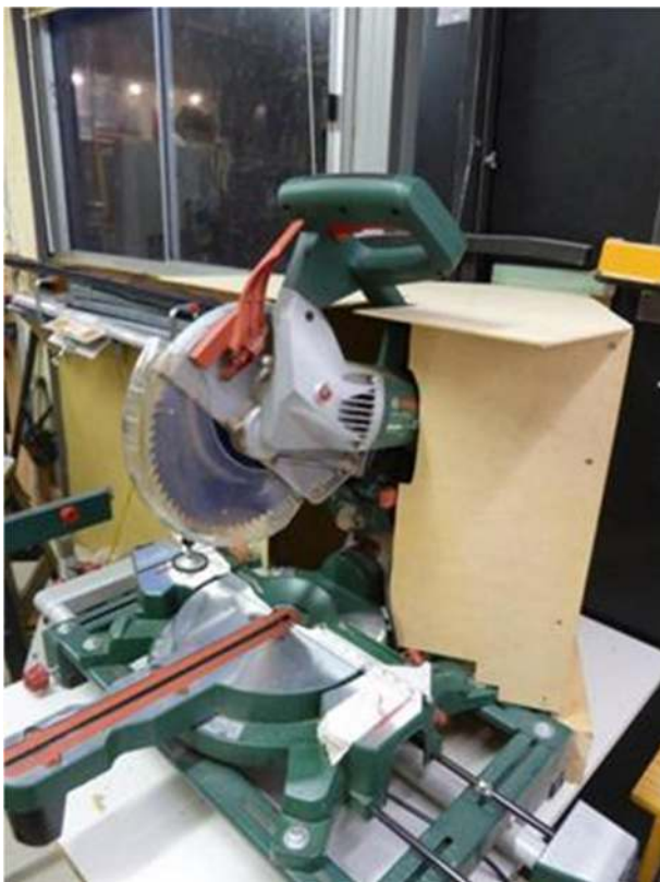
Photo 8: Front faces were cut to fit the mouldings of the saw. They extend forward so the overall shape of the shroud is a diamond. Fortunately these faces were attached with screws because I
