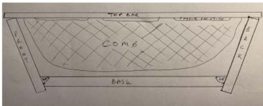
I then created two templates that were used to ensure the front and back boards align to the now  $60^0$  angled bottom board.
