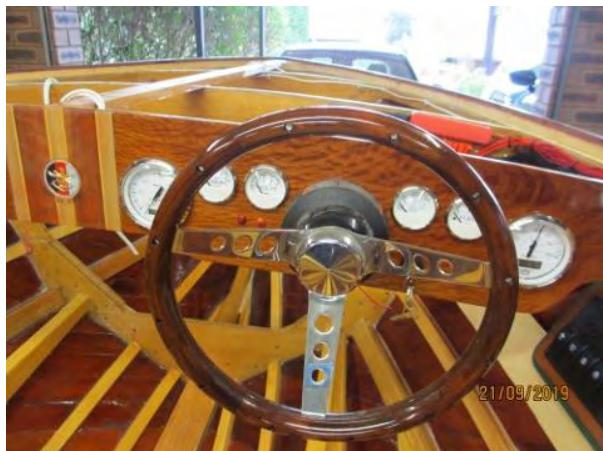
The steering console fitted in October 2019. All of this is magnificent work all taking place in Bob's garage in Canberra. He has aimed to use as much Aussie sourced products as possible using Hoop pine plywood for the double diagonal planking and then Jarrah strips as his finish layer.
