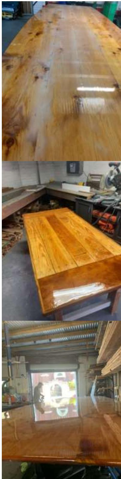
The above photo shows the finished product. Looking pretty good with the roller door open. They decided to leave it as a Bote Coted finish as it came up looking pretty good. The technique used to achieve the great finish was to add 10% metho in the Bote Cote for the last coat so that it goes on like thick varnish. Do not use metho in you coats when building up your waterproof layer as the Epoxy layer will not be thick enough to make it waterproof.
