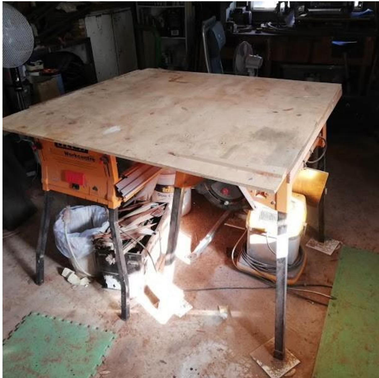
It's slightly fiddly, especially if the tables happen to move, but it's a cheap and effective way of having a central work table which can be accessed from all sides.
