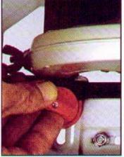
Screw the knobs on (the screws cut their own threads) until they scrape against the top edge of the saw base-plate. Leave the knobs with their cutaway sections facing away from the saw.
