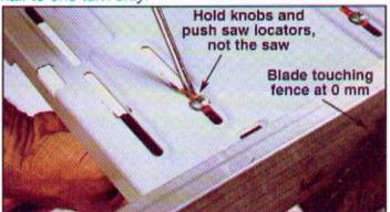
Push the saw locators to move the saw. Do not push the saw itself as this may dislodge the clamps.
