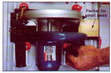
The saw is now set up, and is available at any time for hand-held use by loosening the knobs half a turn and lifting the saw straight up. If the locators are correctly fitted, the saw will go back into exactly the same position each time.
