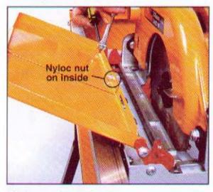
Fit the two longer Philips-head screws (L) through the pivot brackets and the guard flanges and fit the Nyloc nuts. Tighten until the guard is firm, but still free to pivot. Finally, tighten the screw holding the two halves together.
