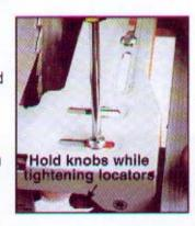
Undo the clamping knobs a couple of turns and check that you cannot move the saw baseplate sideways at all between the locators.
