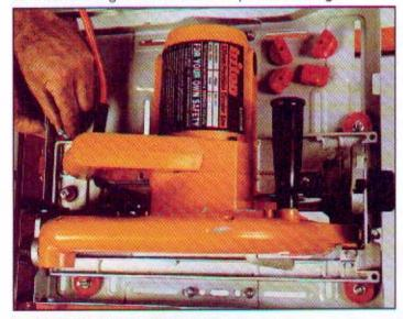
Fitting the saw locators and knobs
