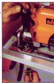
Screw the knobs on (the screws cut their own threads) until they just scrape against the top edge of the saw base-plate. This will hold the saw upside-down for final adjustment, and still allow it to be shifted sideways using the alignment cams. Leave the knobs
