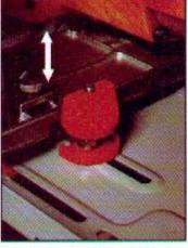
Turn the saw right-way up again and loosen the four knobs a couple of turns. Push the saw sideways to ck that it cannot move, and that all screws are turny tightened. Do up the knobs again, perhaps one turn beyond when they first scrape on the baseplate.
